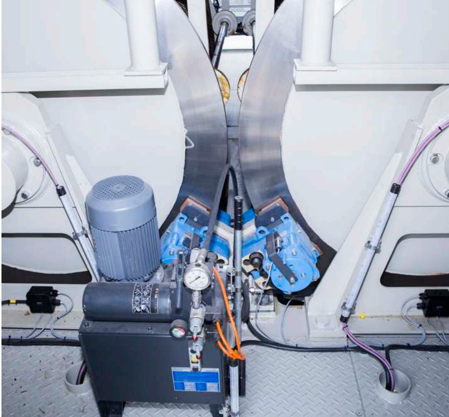
↑ Safety brakes on the lifting gear
